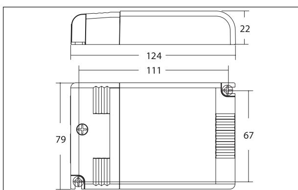
Powerful all-in-one converter, with inbuilt PWM dimmer, for LEDs. Ready, after a simple installation, to drive most types of LED light sources, both constant voltage DC (48V) and constant current DC (350, 500, 550, 650, 700, 750, 850, 900, and 1050 mA). 1-10 units can be interconnected and controlled from one or more locations using momentary push-buttons via potentiometers, 1-10V or a bus/KNX system via actors. 15 cm sync cable included.
